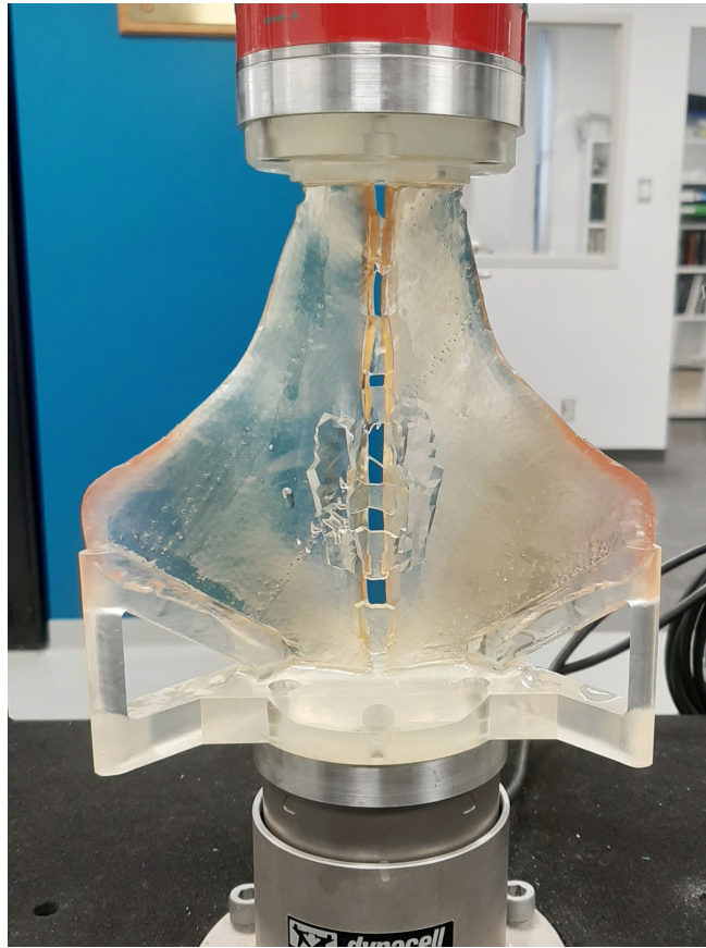
Developed tlf analogue mounted on custom tensile jig.jpeg
